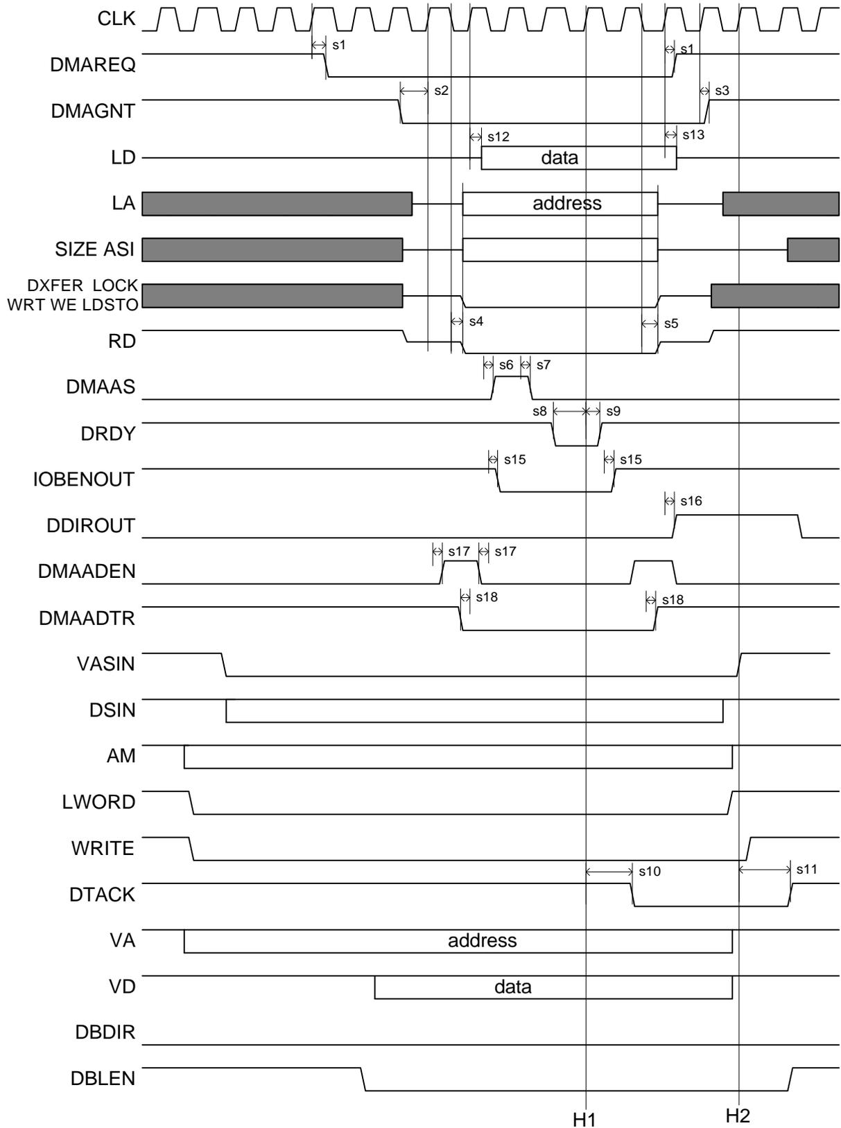
Figure 2.5-16 EVI slave : VME single write access
