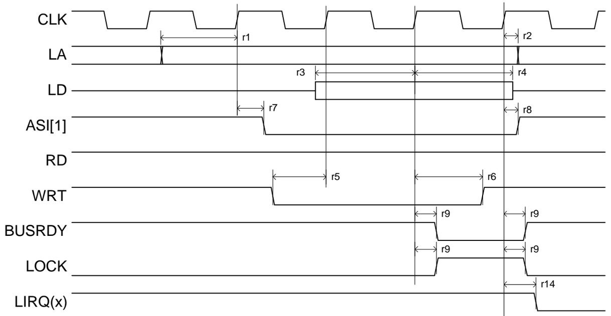
Figure 3.5-1 EVI Register write
