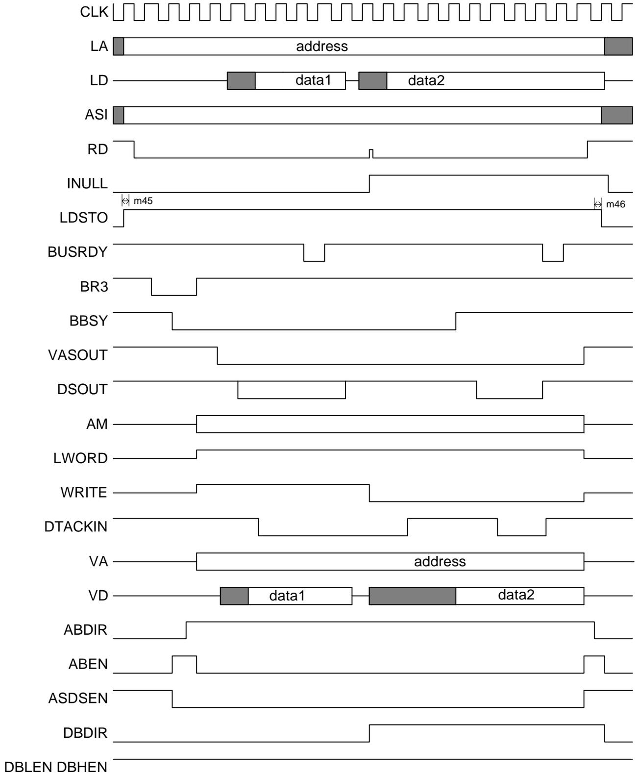
Figure 2.5-6 : EVI master : VME read modify write issued from an ERC load store instruction
