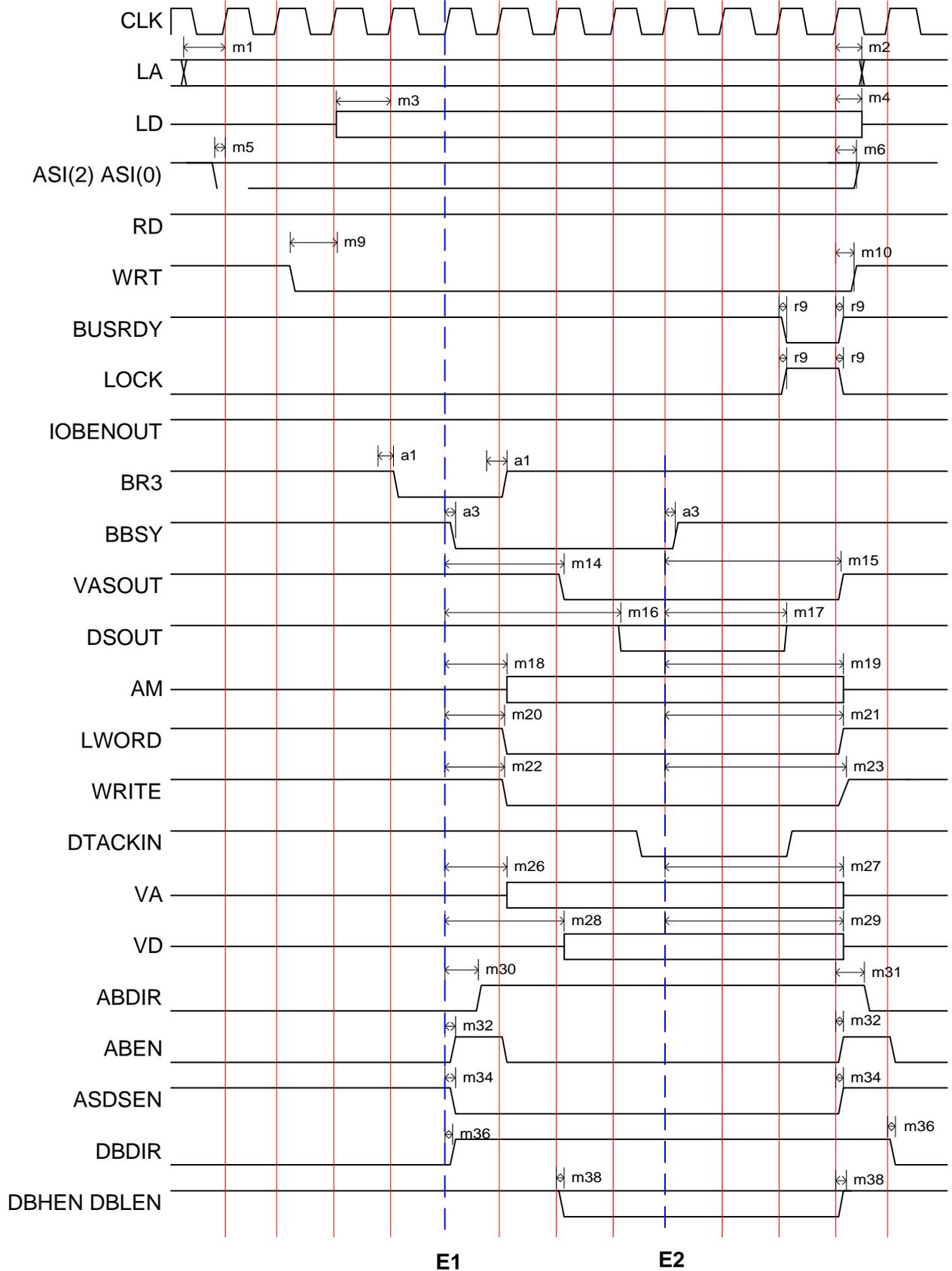
Figure 3.5-3 EVI Master : single access write
