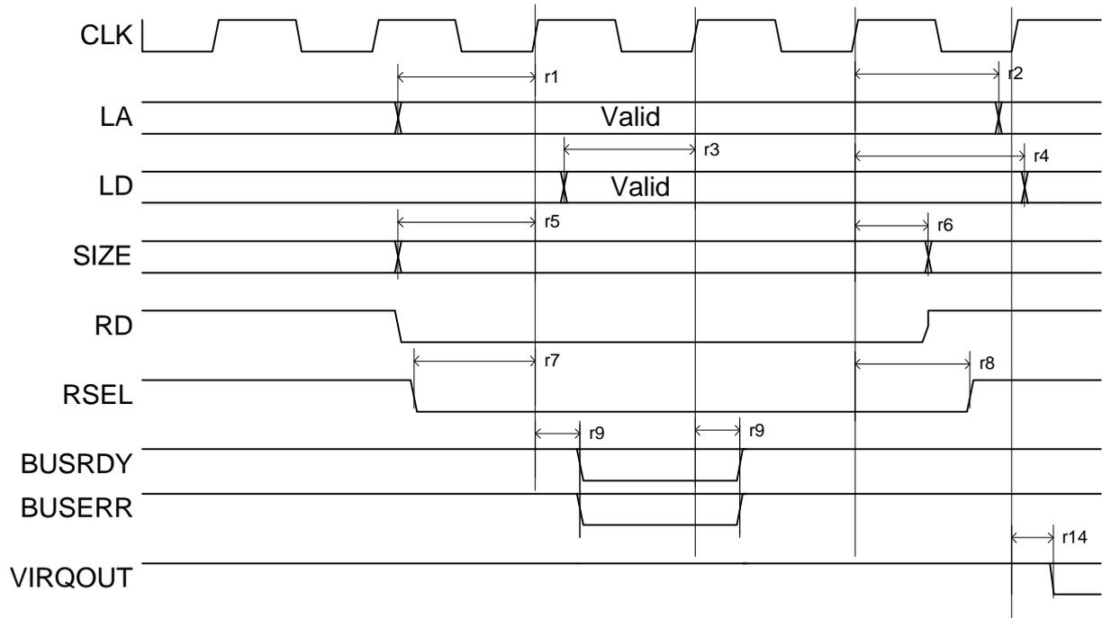
Figure 2.5-1 EVI Register write
