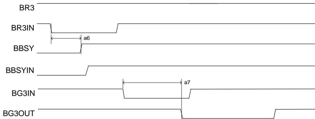
Figure 2.5-11 EVI32 not Arbiter - Daisy chain propagation
