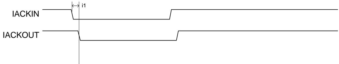
Figure 2.5-12 IACK daisy chain propagation
