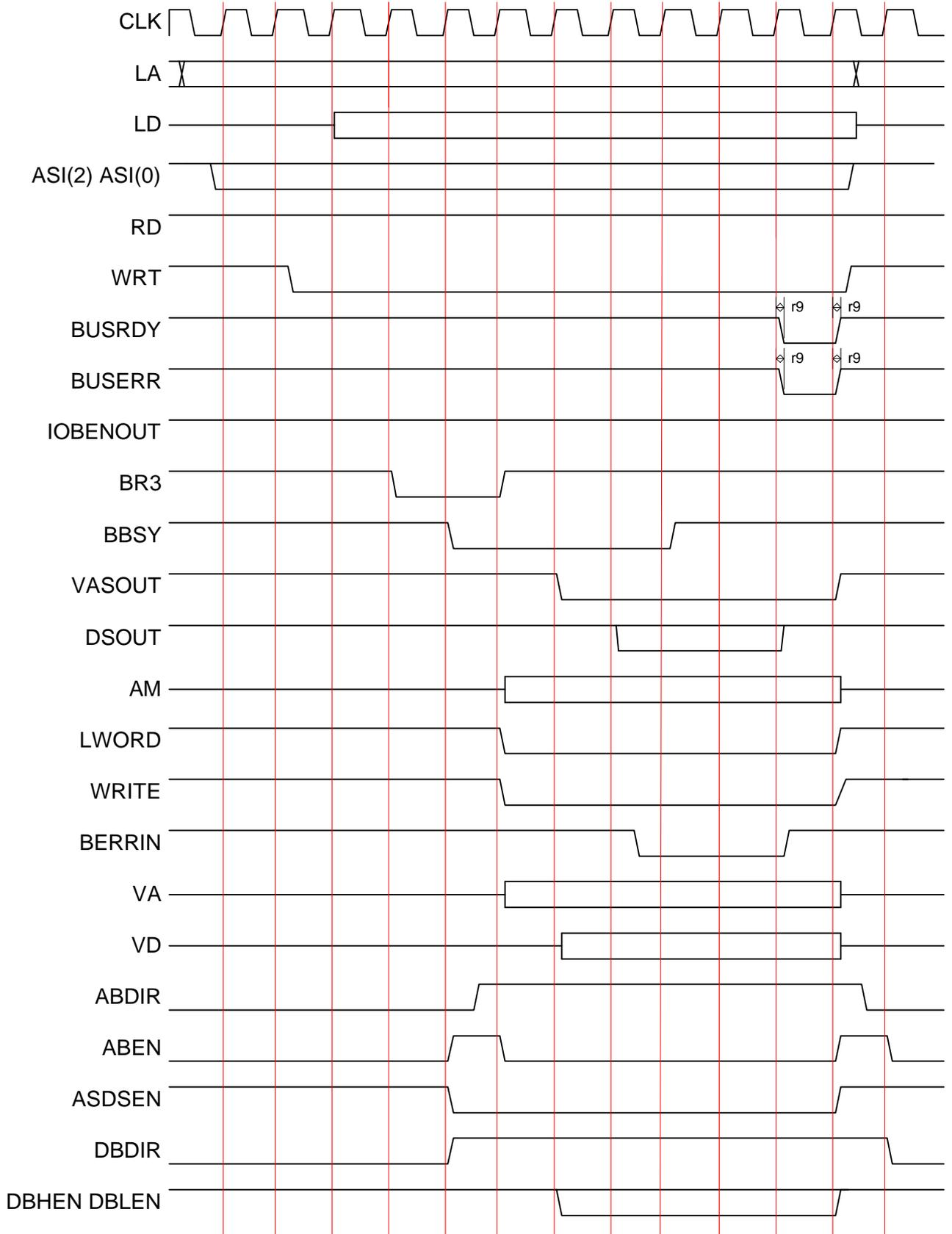
Figure 3.5-5 : EVI Master : access ending by a BERR
