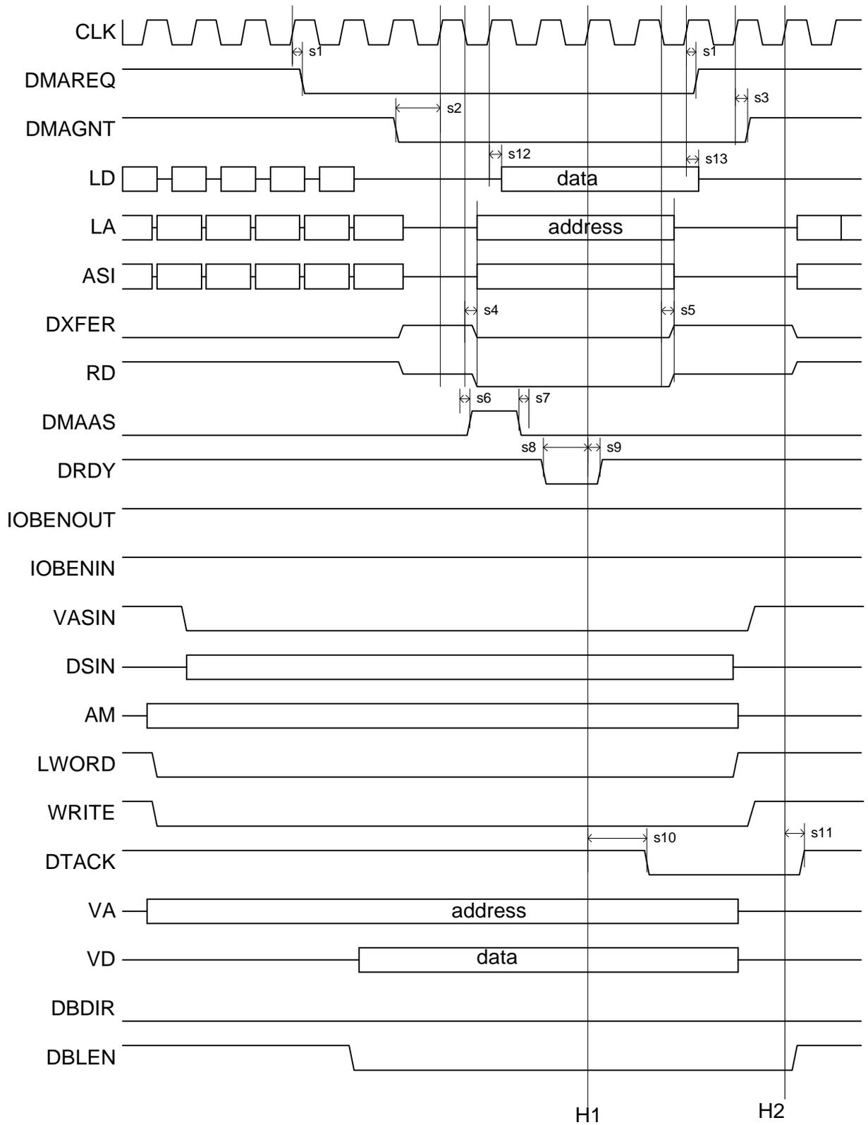
Figure 2.5-21 ERC32 3C - EVI slave : VME single write access
