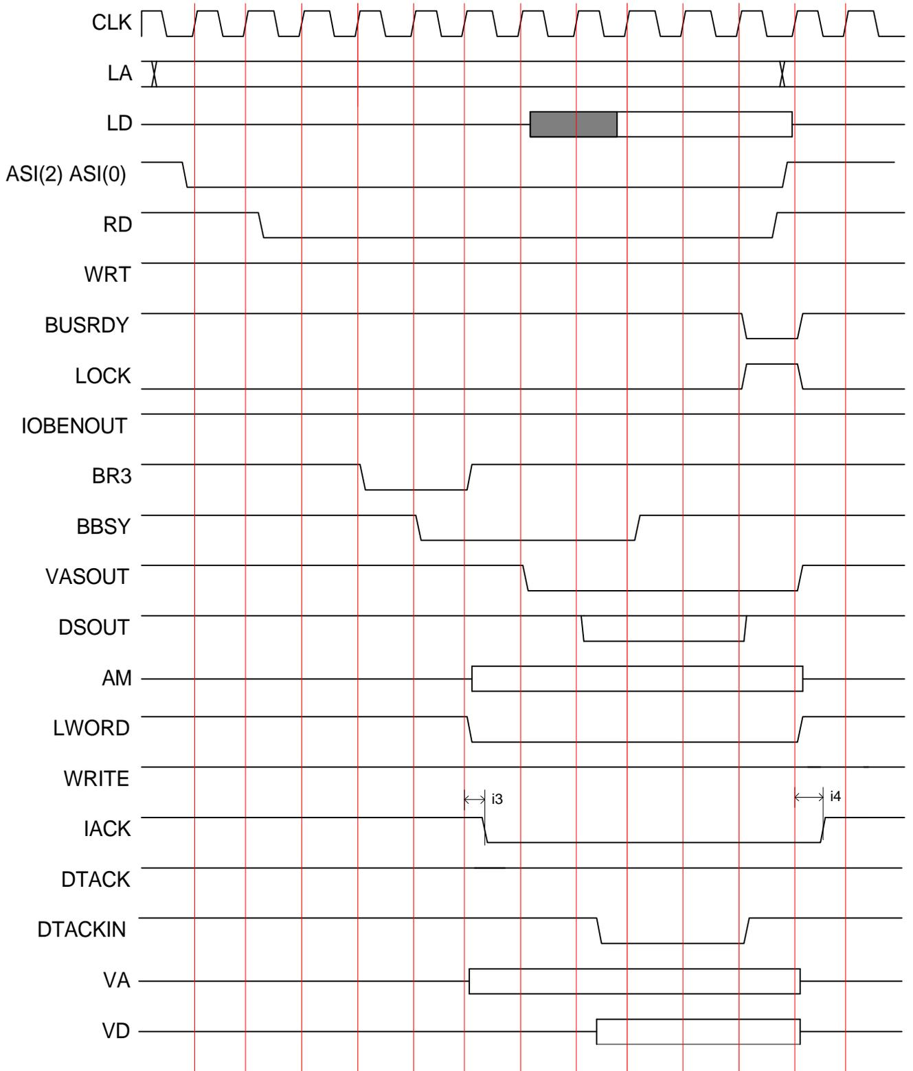
Figure 3.5-11 EVI interrupt acknowledge cycle
