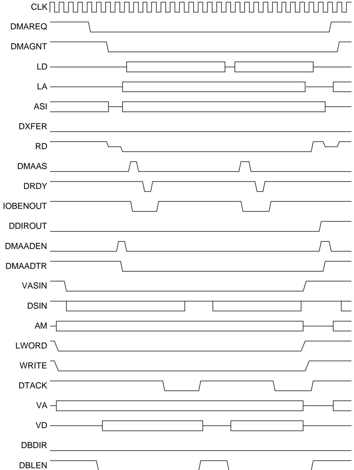
Figure 2.5-17 EVI slave : VME Block transfer write access
