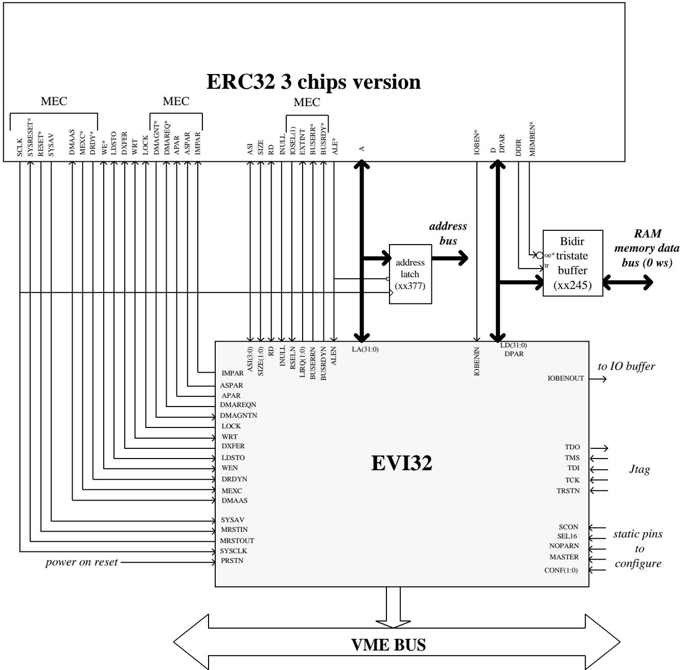
Figure 2.3-2 – ERC/3C - EVI interface drawing
