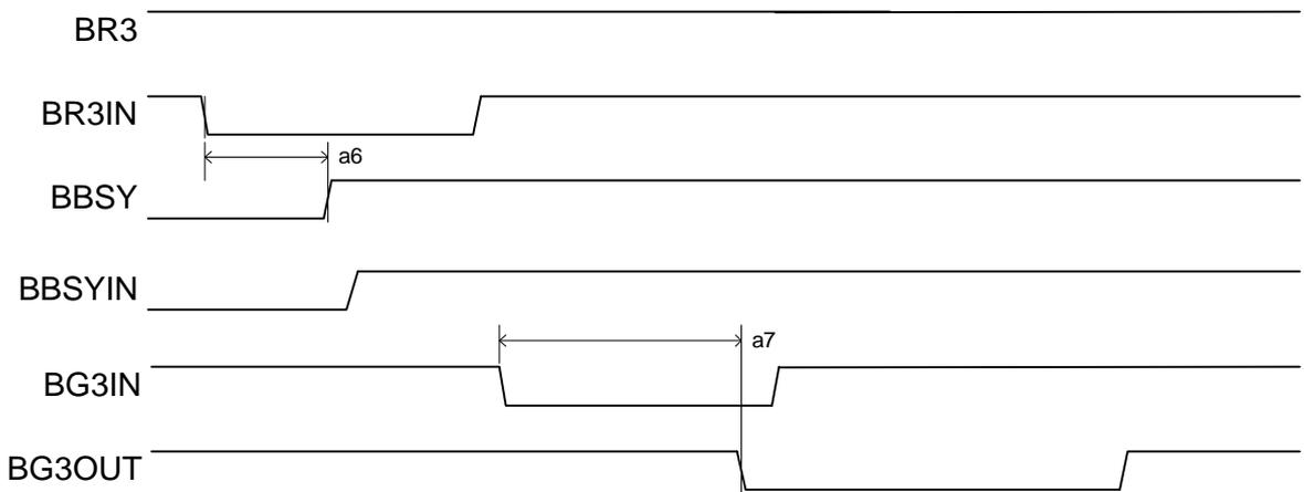
Figure 3.5-8 EVI32 not Arbiter - Daisy chain propagation
