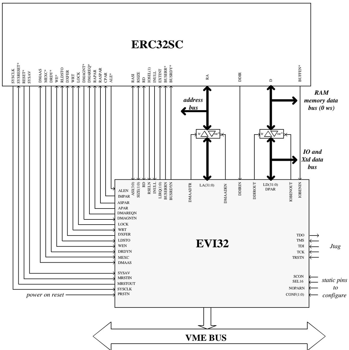
Figure 2.3-1 – ERC/SC - EVI interface drawing
