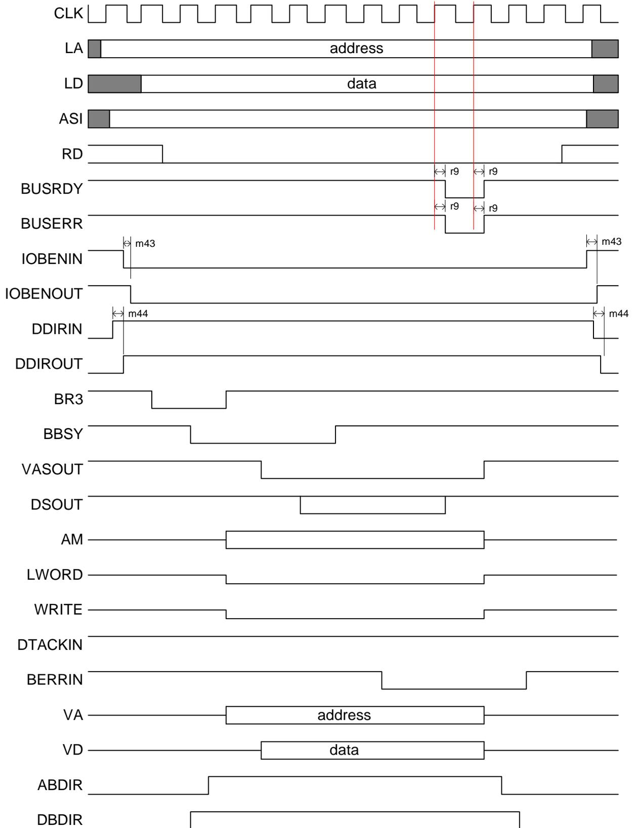
Figure 2.5-5 : EVI Master : access ending by a BERR
