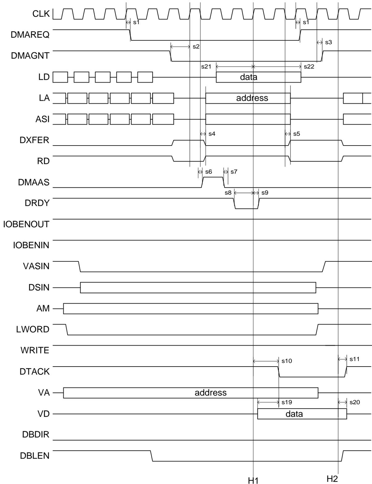
Figure 2.5-20 – ERC32 3 chips - EVI slave : VME single read access
