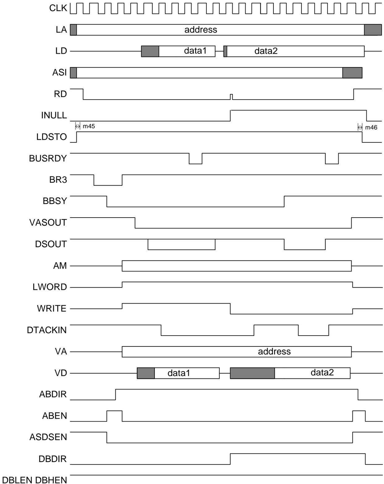
Figure 2.5-18 : ERC32 3C - EVI master : VME read modify write issued from an ERC load store instruction
