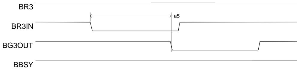
Figure 2.5-10 EVI Bus Arbiter - EVI32 as Arbiter initiating Arbitration daisy chain
