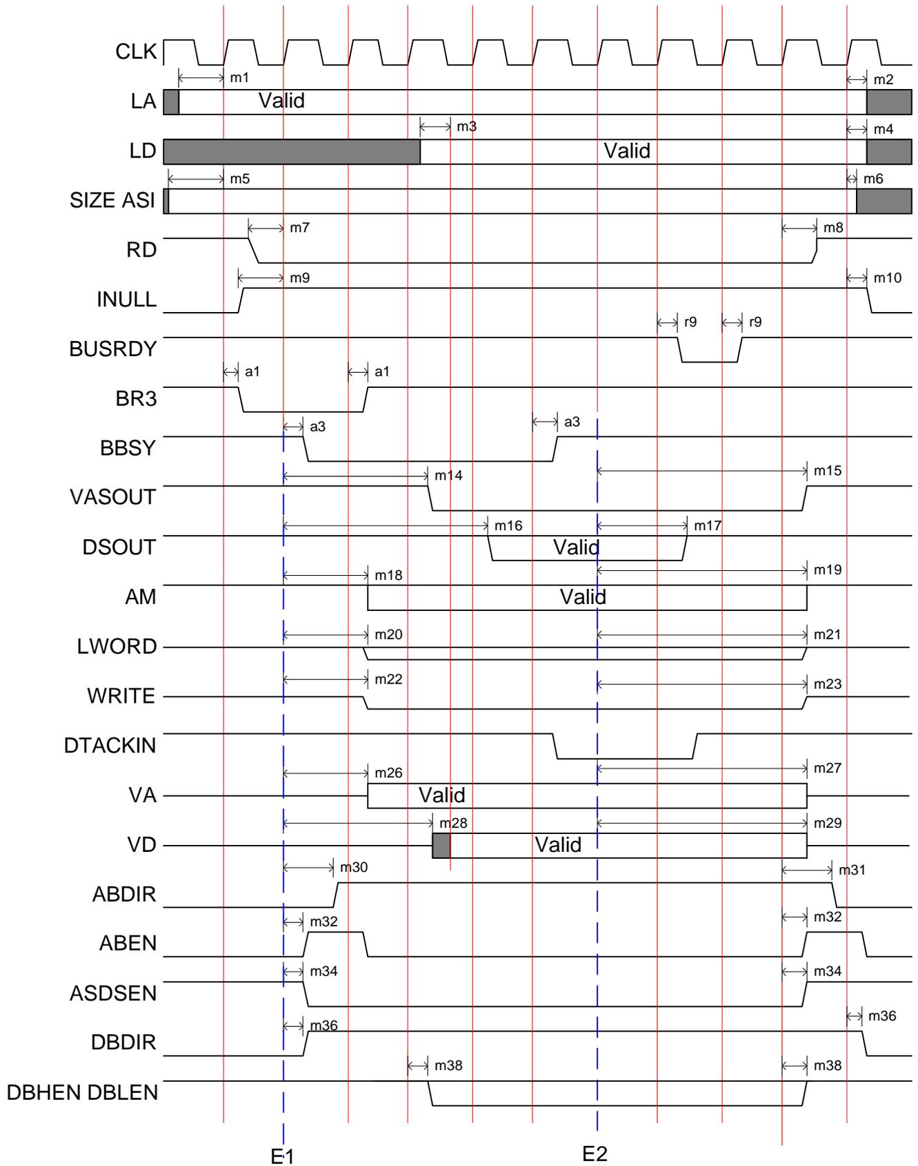
Figure 2.5-3 EVI Master : single access write
