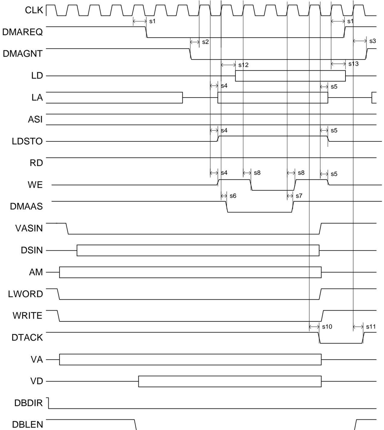
Figure 3.5-13 EVI slave : VME single write access
