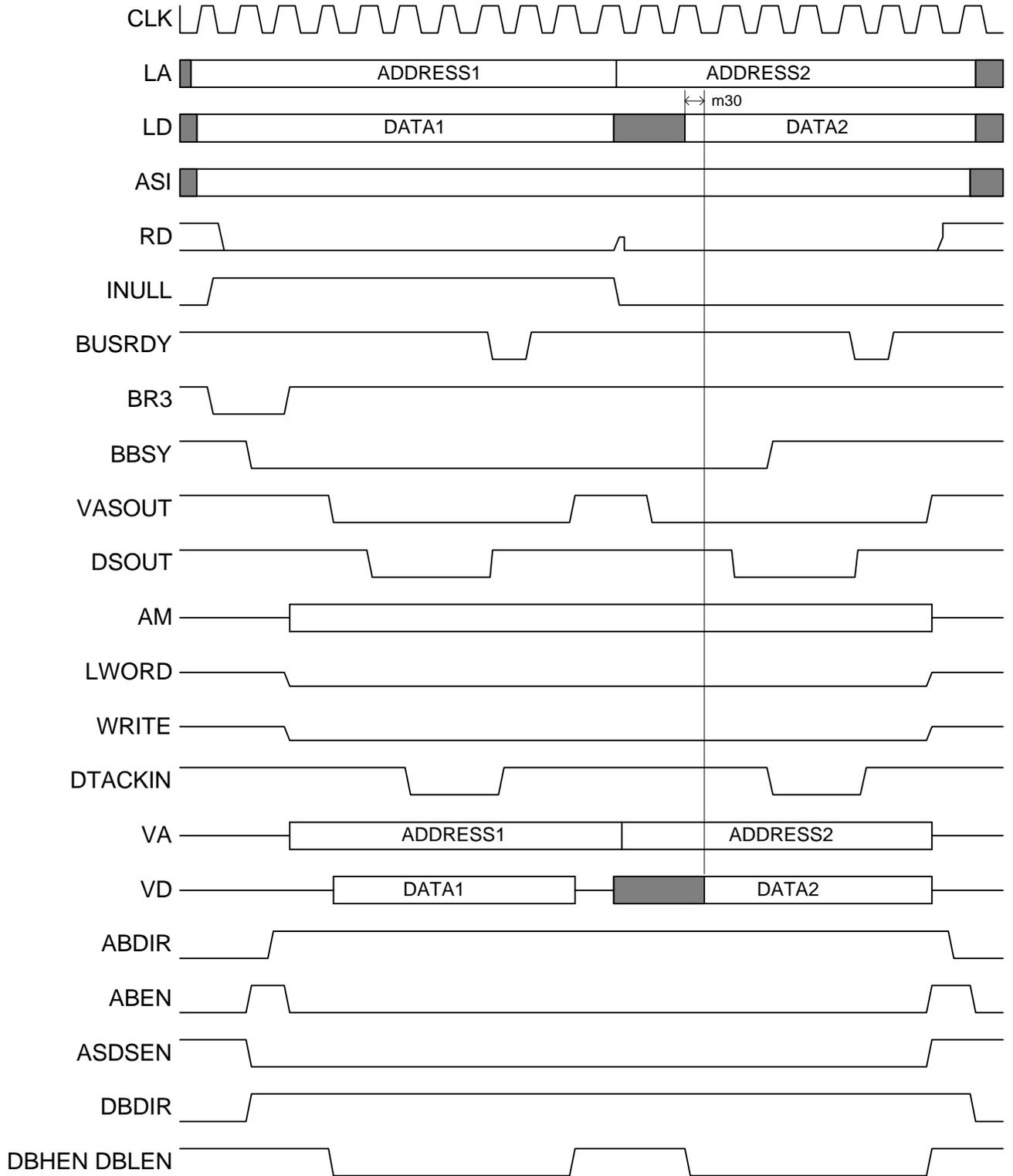
Figure 2.5-7 - EVI Master : double VME write from an ERC32 Store Double instruction
