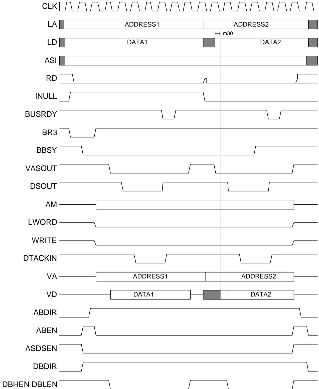
Figure 2.5-19 – ERC32 3C - EVI Master : double VME write from an ERC32 Store Double instruction
