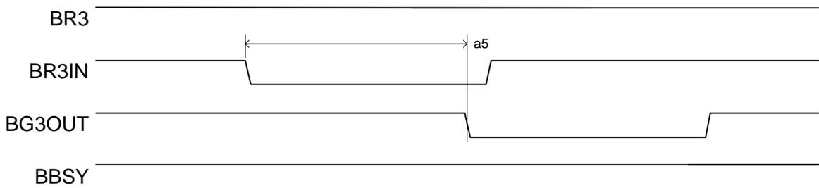
Figure 3.5-7 EVI Bus Arbiter - EVI32 as Arbiter initiating Arbitration daisy chain
