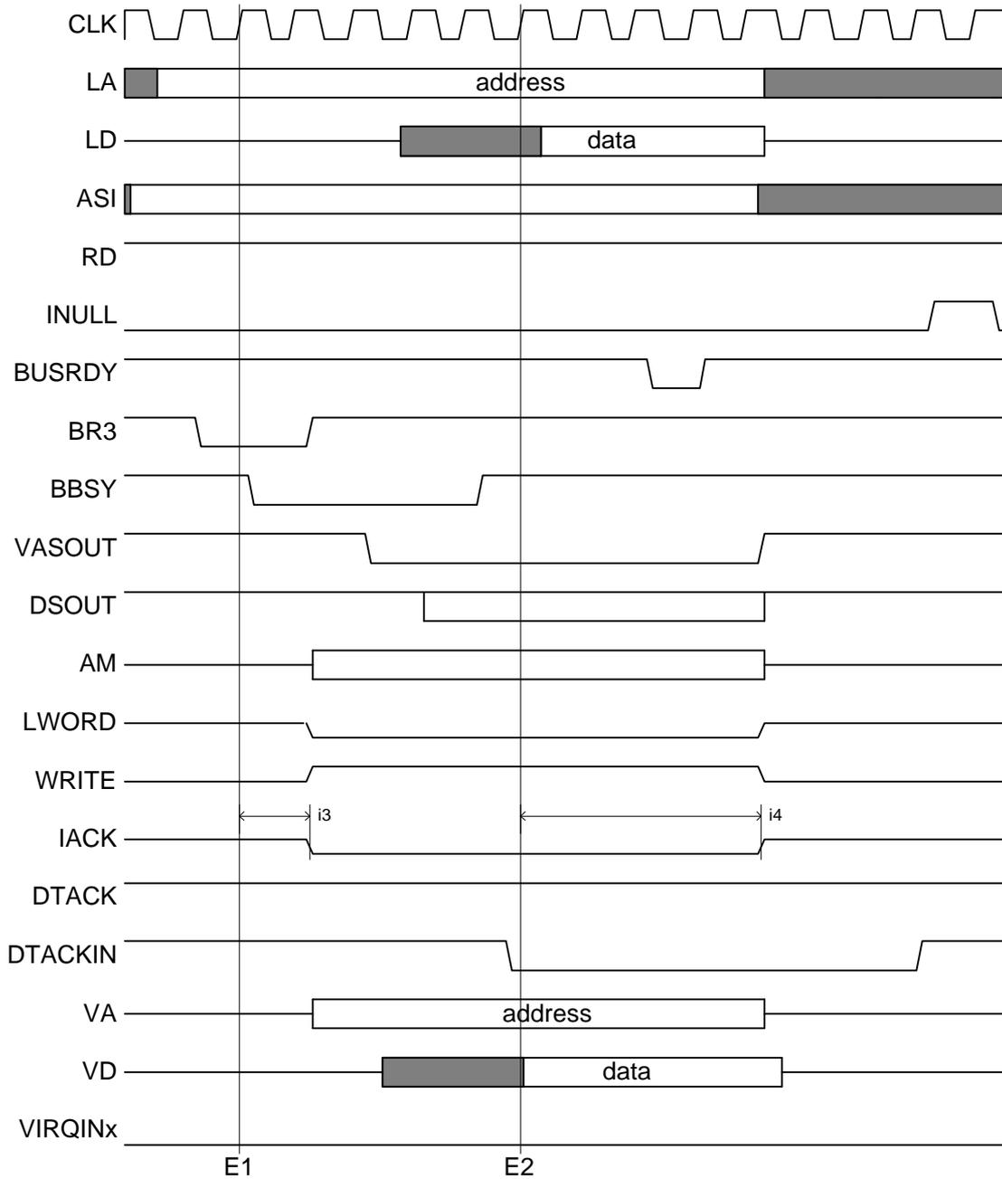
Figure 2.5-14 VME Interrupt Acknowledge cycle
