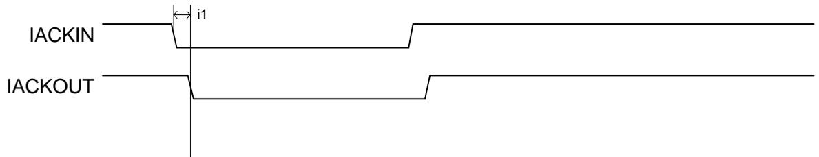
Figure 3.5-9 IACK daisy chain propagation
