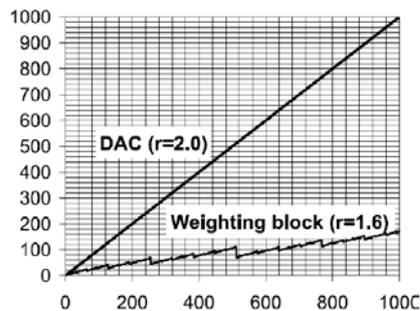
Figure 3-5 Ideal transfer curves of a DAC and of a non-linear weighting block with  $r=1.6$
