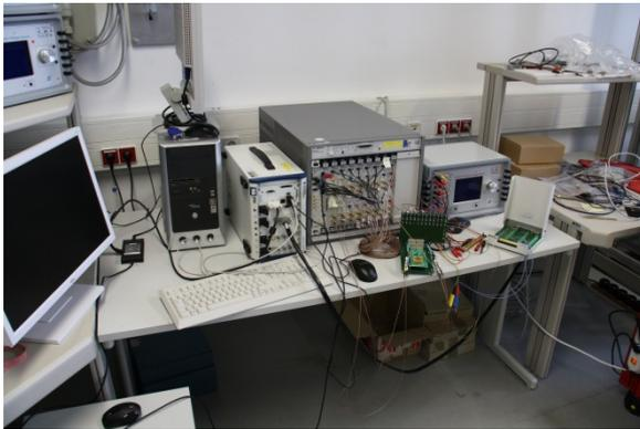
Figure 4-2 Test set-up with a packaged chip test board
