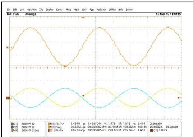
Figure 4-11 The DAC differential outputs at 100 MHz 12-bit sinusoidal signal
