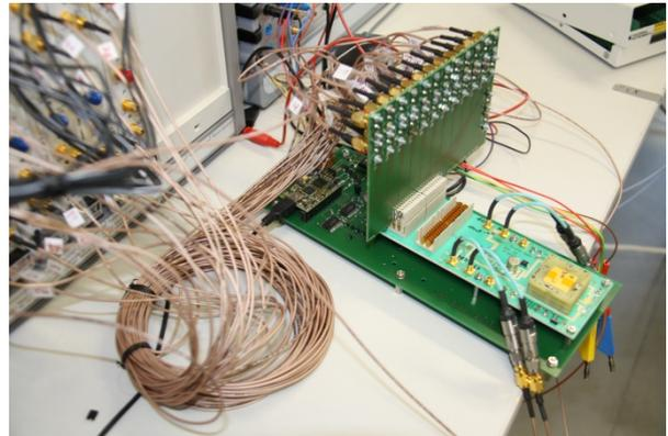
Figure 4-3 A packaged chip test board
