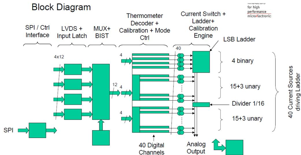
Figure 3-6 Detailed block diagram of the DAC architecture
