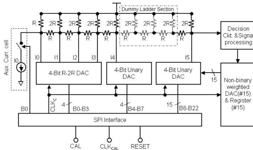
Figure 3-2 Implemented 12-bit architecture ( $B_0$ - $B_3$  = LSBs), ( $B_4$ - $B_{11}$  = MSBs)
