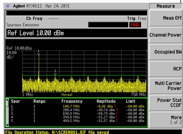
Figure 4-12 SFDR measurement at 100 MHz sinusoid
