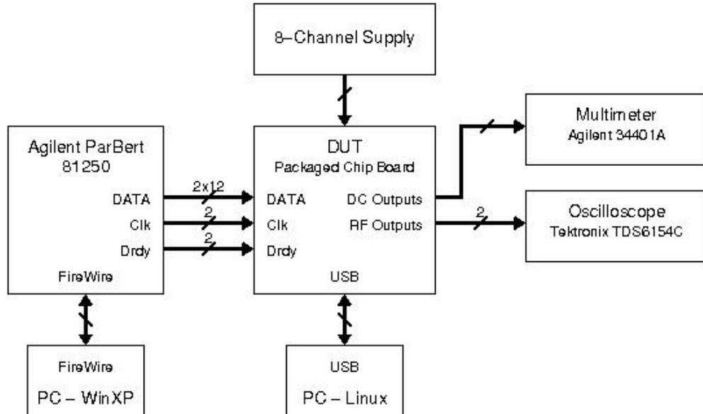
Figure 4-1 General test set up for dynamic and static testing of the high speed part by using the packaged chip board
