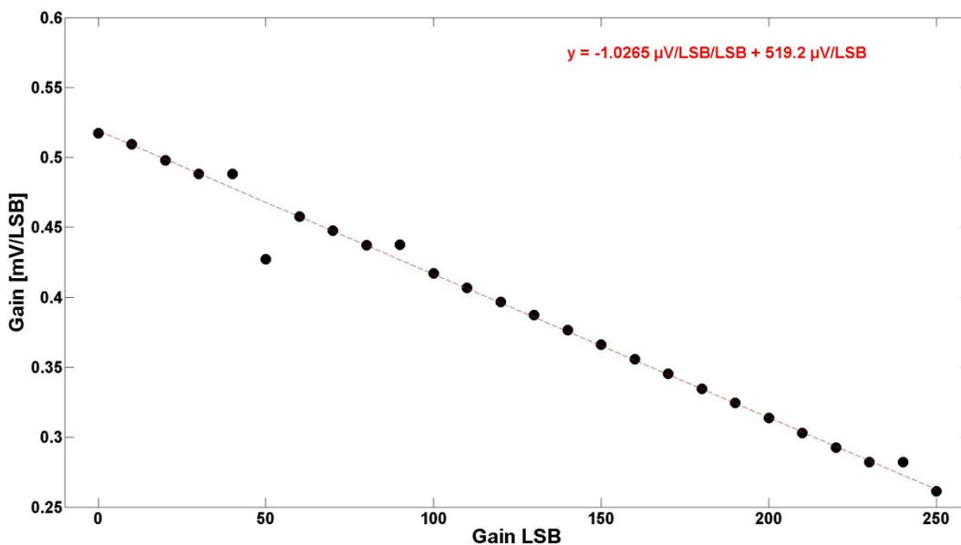
Figure 4-8 Measured and fitted DAC gain in dependency of the gain setting
