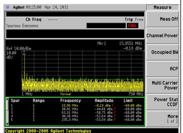
Figure 4-14 SFDR measurement at 143 MHz sinusoid
