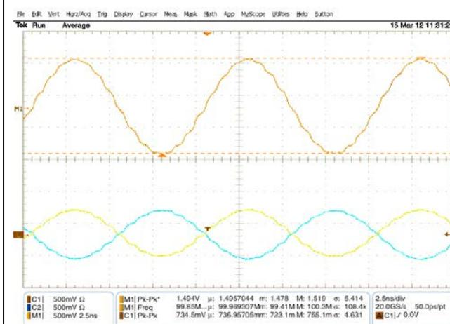
Figure 4-15 The DAC differential outputs at 340 MHz 12-bit sinusoidal signal
