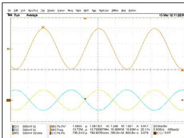
Figure 4-9 The DAC differential outputs at 15 MHz 12-bit sinusoidal signal
