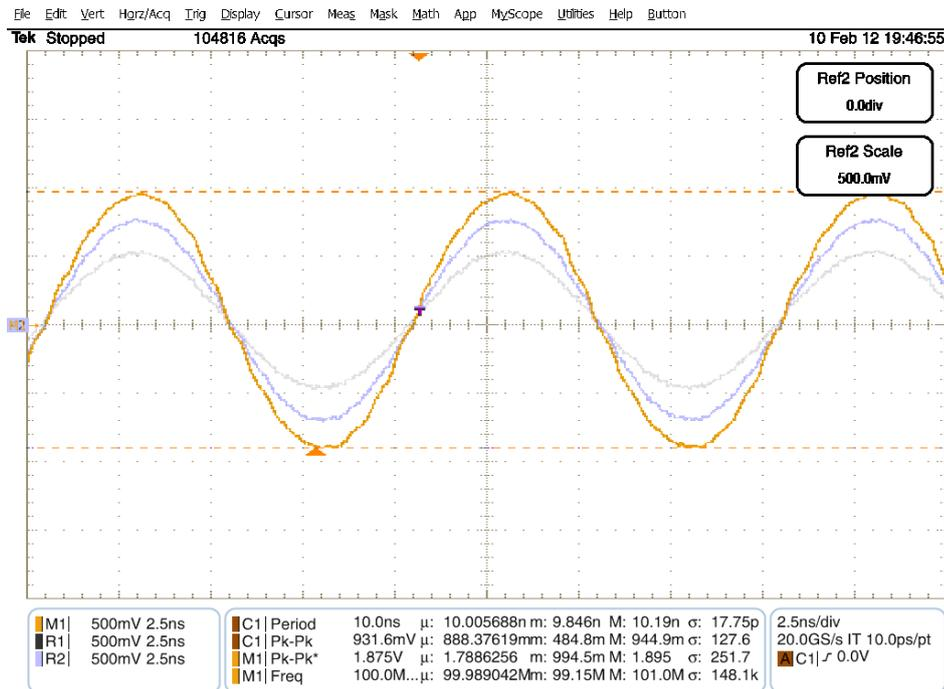
Figure 4-6 DAC output differential voltage at three gain values of 0x00, 0x80, and 0xFF
