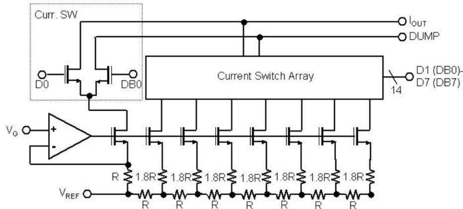
Figure 3-4 Block diagram of 8-bit non-binary weighted DAC
