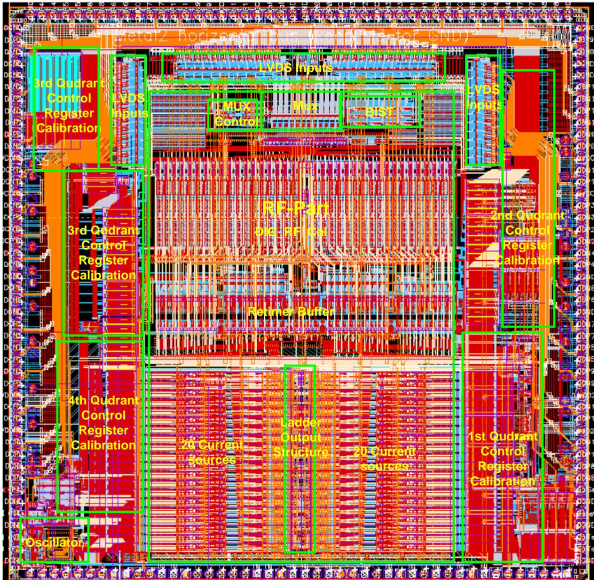
Figure 3-7 Final full chip layout (filler structures not shown)
