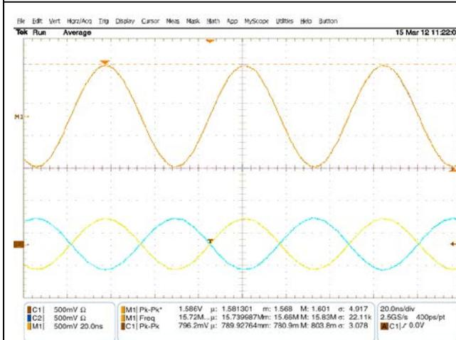
Figure 4-13 The DAC differential outputs at 143 MHz 12-bit sinusoidal signal
