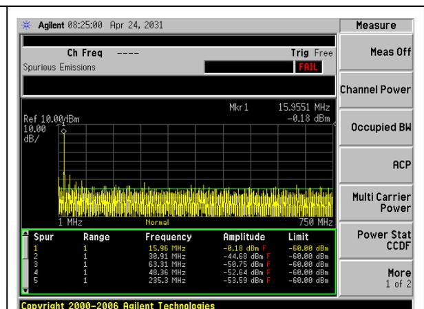
Figure 4-10 SFDR measurement at 15 MHz sinusoid
