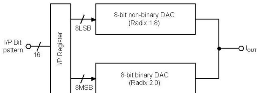
Figure 3-3 Block diagram of 16-bit non-binary weighted DAC
