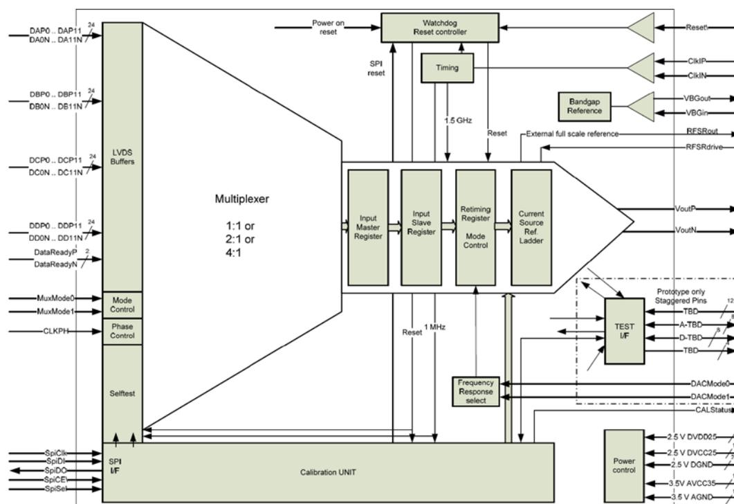
Figure 3-1 Functional block diagram of the 12 Bit 1.5GSps DAC
