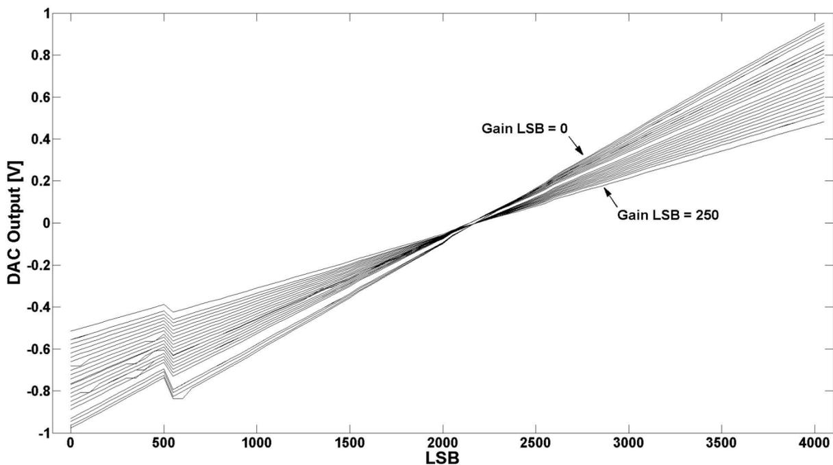
Figure 4-7 Measured DAC output ramps with varies gain settings
