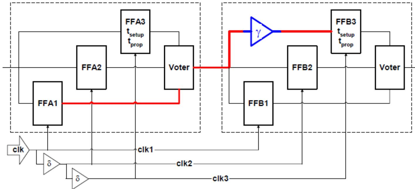
**Automatic buffer insertion by fix-hold of synthesis tool compensates clock skew → and spoils SET protection**
