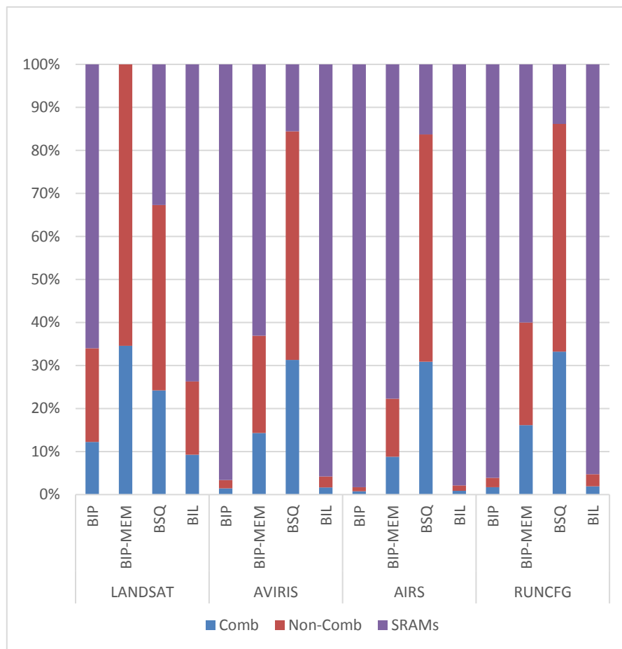
Figure 2-14: CCSDS-123 DARE 180nm mapping: area distribution (*)
